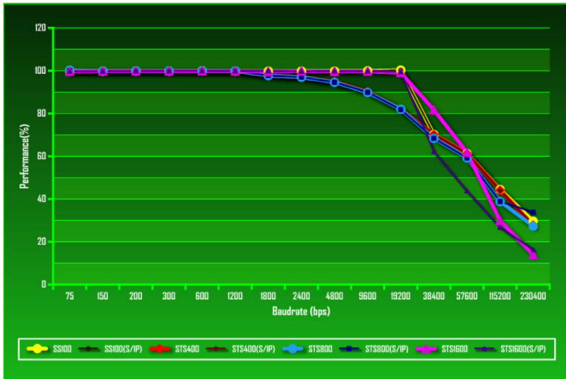
Figure 10: Throughput Test Result of Super Series and STS Series – TCP/IP vs. Serial/IP Bluetooth-Serial Adapters
