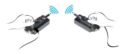
Parani-SD provides Pairing Button for instant configuration without a PC to make an automatic connection between two Parani-SDs. (Two Parani-SDs as SD1 and SD2, respectively.)
