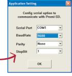
Parani-FSD Series default configuration is 9600 bps Baud rate. 8 Data bits. No Parity. 1 Stop bit and H/W flow control
