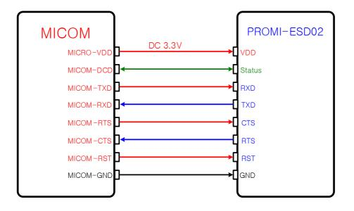
**u** When TTL level of MICOM is 3.3V and not using hardware flow control
