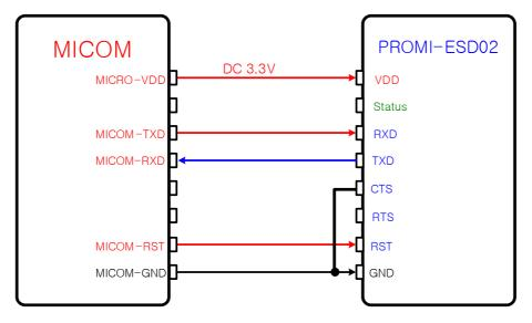
aggregation When TTL level of MICOM is 5V
