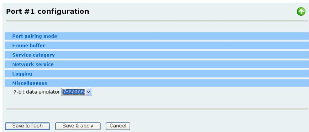
The image shows a configuration window titled "Port #1 configuration". It contains several menu items: "Port pairing mode", "Frame buffer", "Service category", "Network service", "Logging", and "Miscellaneous". The "Miscellaneous" menu is selected and expanded, showing a "7-bit data emulator" dropdown menu with "7-space" selected. At the bottom of the window, there are three buttons: "Save to flash", "Save & apply", and "Cancel".
