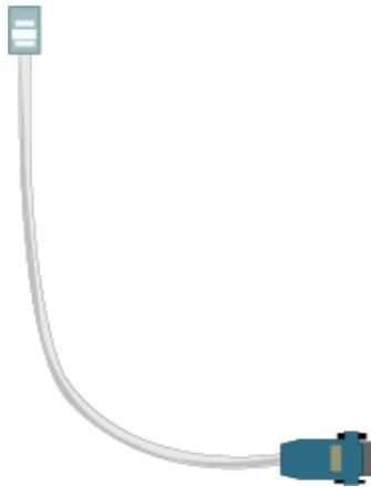
Console cable + RJ45-DB9F adapter
