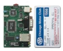
The small size of the 1300 board can be easily embedded in a parent device.
